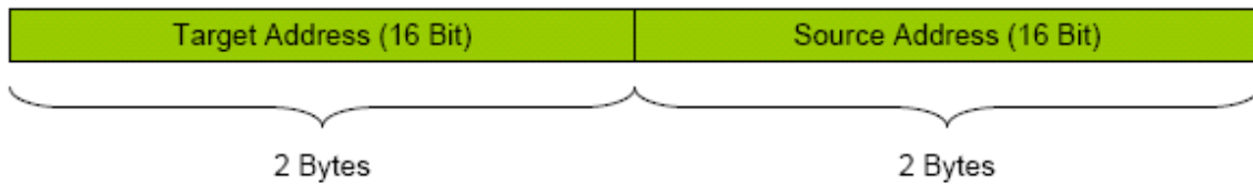
Figure 15: Address header for 2 Byte addressing
