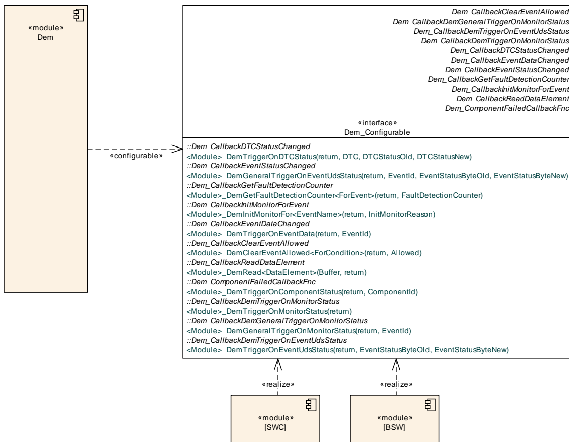
Figure 8.4: Configuration interfaces of the Dem module
