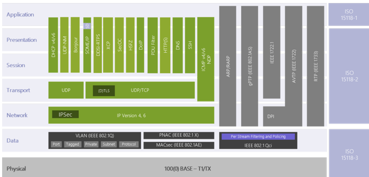
Figure 4.1: Protocols related to Ethernet in ISO/OSI layers
