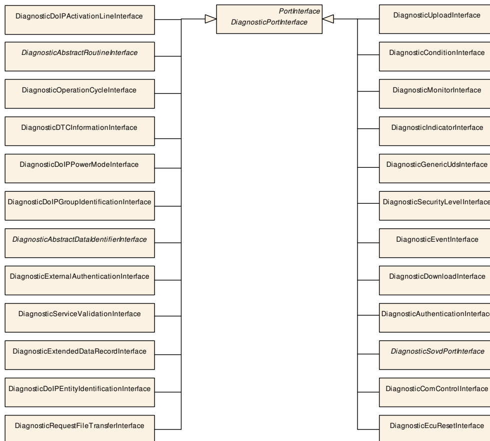
Figure 4.31: Modeling of PortInterfaces for diagnostic purposes
