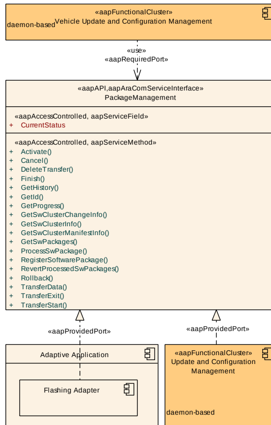
Figure 9.99: Interfaces required by Vehicle Update and Configuration Management (part 3)
