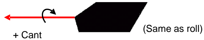
Figure 2.4: Plus, or minus sign of cant
