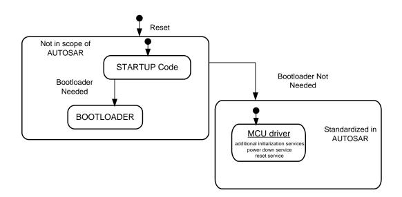
The MCU driver accesses the microcontroller hardware directly and is located in the Microcontroller Abstraction Layer (MCAL).
