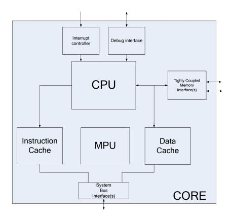
The requirements are derived from the automotive standards. Busses have to be tested including arbitration, MMU/MPU, caches, tightly coupled memories, general purpose and dedicated registers, numerical execution units, including address generation and interrupts plus exception handling.
