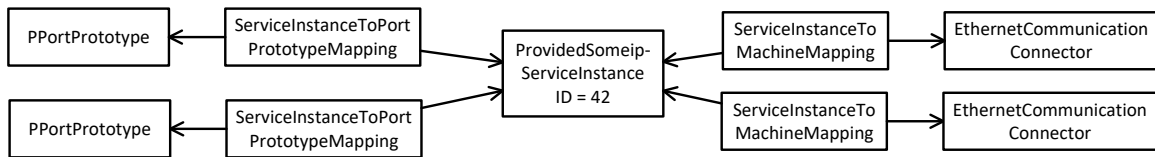
Figure 11.13: Scenario in which a ProvidedSomeipServiceInstance is provided on two VLANs and is mapped to different PPortPrototypes from which latest at runtime only one is operational
