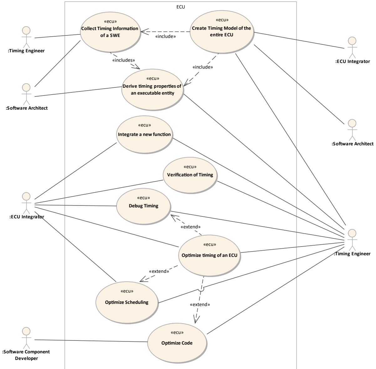
Figure 7.2: Use case diagram: Timing Analysis for ECU
