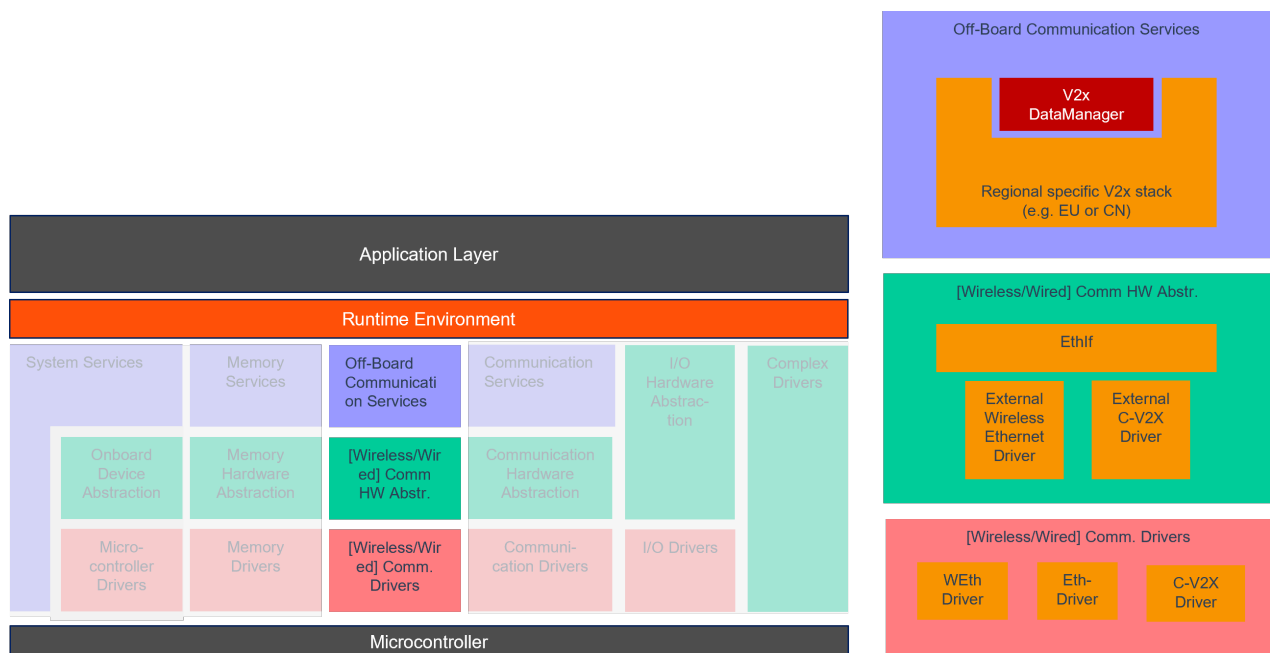
Figure 7.1: AUTOSAR layered view with V2xDM
