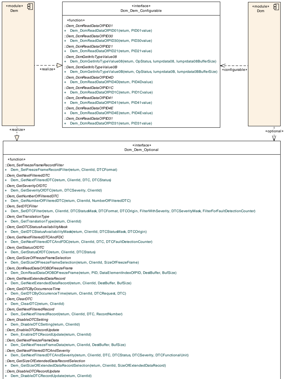
Figure 8.3: Overview of interfaces between the Dem and Dcm
