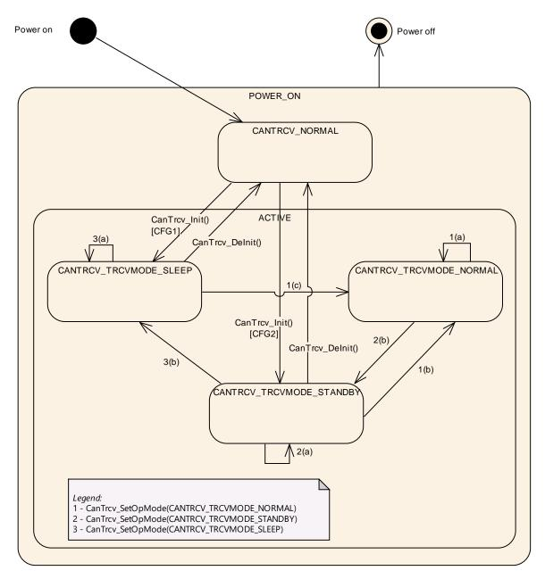
The main idea intended by this diagram, is to support a lot of up to now available CAN bus transceivers in a generic view. Depending on the CAN transceiver hardware, the model may have one or two states more than necessary for a given CAN transceiver hardware but this will clearly decouple the ComM and EcuM from the used hardware.
