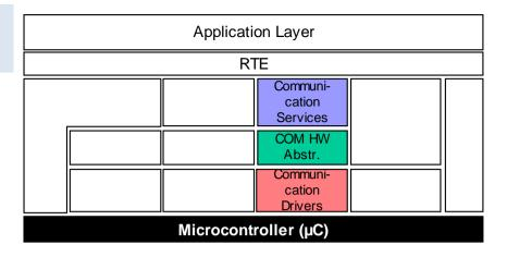
The FlexRay Communication Services are a group of modules for vehicle network communication with the communication system FlexRay.
