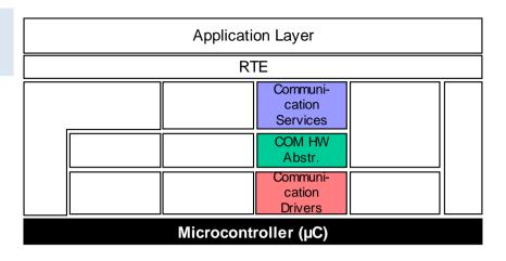
The TCP/IP Communication Services are a group of modules for vehicle network communication with the communication system TCP/IP.
