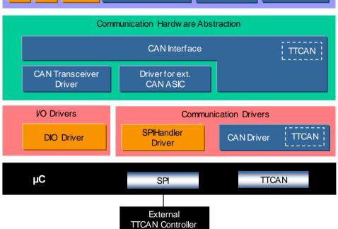
The **TTCAN Communication Services** are the optional extensions of the plain CAN Interface and CAN Driver module for vehicle network communication with the communication system TTCAN.
