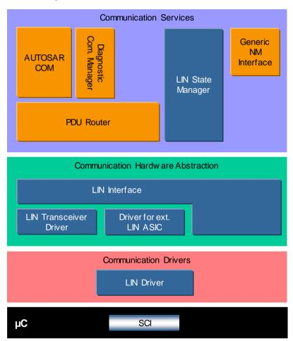
The **LIN Communication Services** are a group of modules for vehicle network communication with the communication system LIN.
