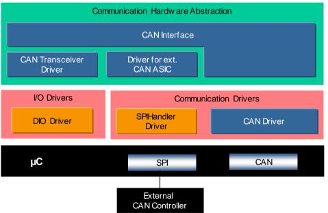
The **J1939 Communication Services** extend the plain CAN communication stack for vehicle network communication in heavy duty vehicles.
