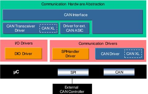
The CAN Communication Services are a group of modules for vehicle network communication with the communication system CAN.
