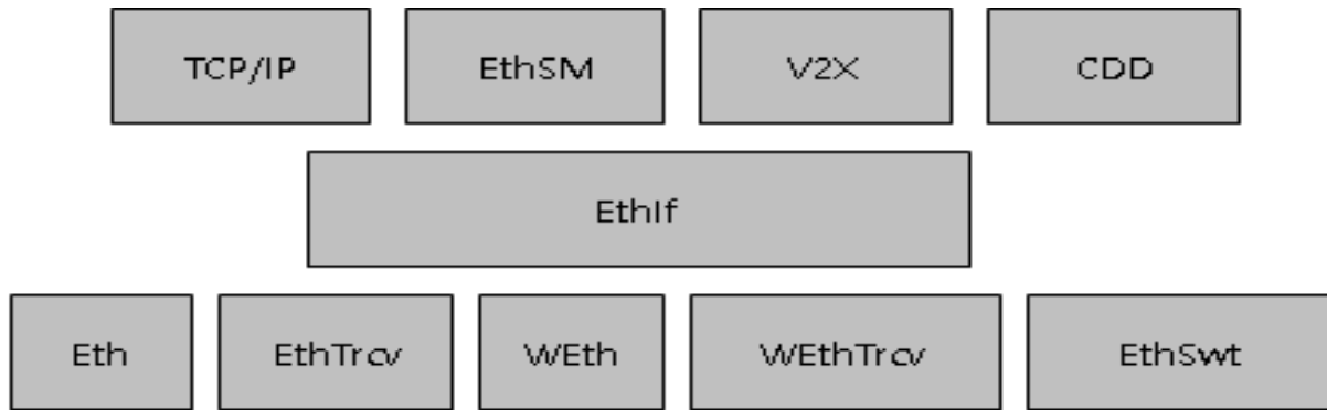
Figure 1: Ethernet stack module overview
