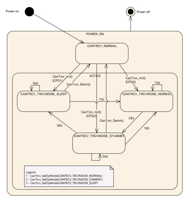
The main idea intended by this diagram, is to support a lot of up to now available CAN bus transceivers in a generic view. Depending on the CAN transceiver hard-ware, the model may have one or two states more than necessary for a given CAN
