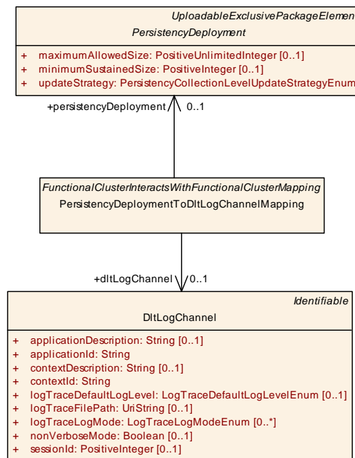
Figure 12.8: Mapping of PersistenceDeployment to DltLogChannel
