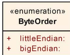
Figure 2: Enumeration to indicate byte order of a processing unit.
