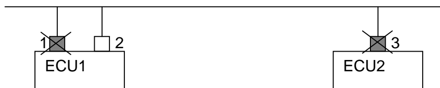
Figure 41: Example for a forbidden Signal Path
