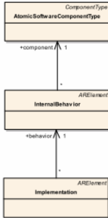
Figure 83: An implementation is associated with a single atomic software component.
