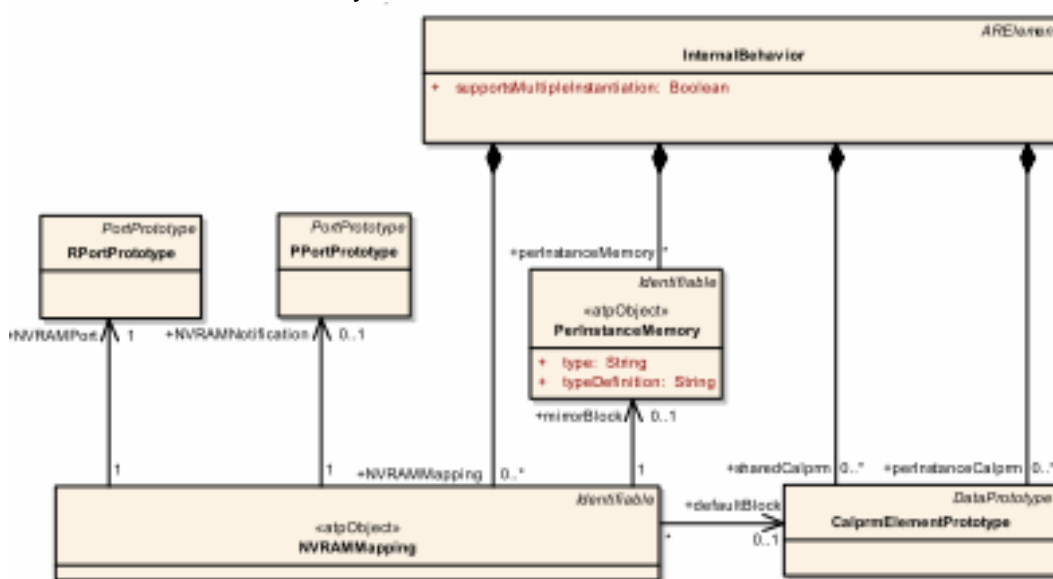
Figure 76: NvRam Manager usage of Per Instance Memory
