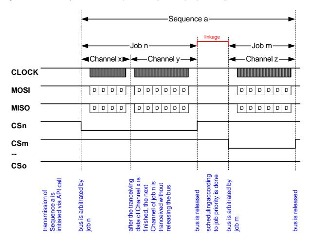
Channels data may differ from the hardware handled and user (client application) given. On the client side the data is handled in 8, 16 or 32bits mode (see chapter 8.2.5). On the microcontroller side, the hardware may handle between 1 and 32bits or may handle a fixed value (8 or 16bits) and this width is configurable for each Channel (see SPI\_DATA\_WIDTH).
