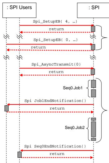
Setup a Channel; initialize buffer pointers and length synchronously. Parameters are saved.
