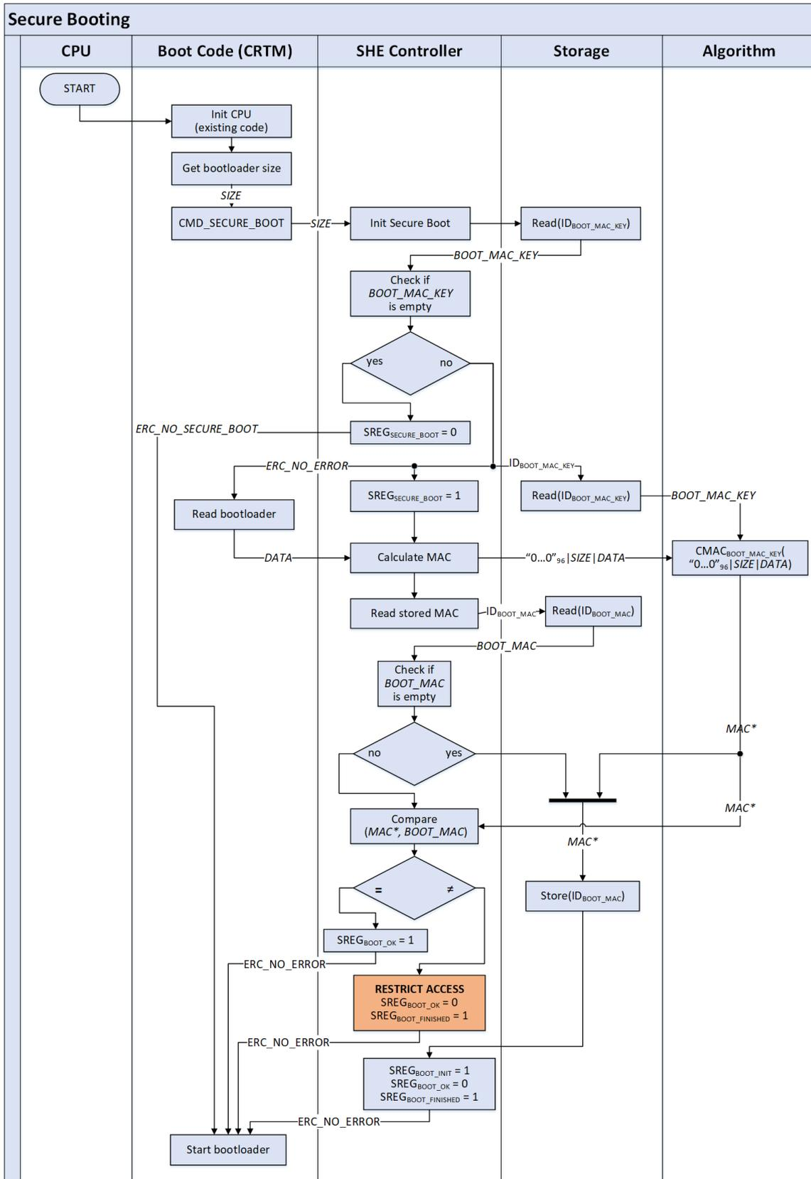
Figure 4.9: Flow chart of the secure boot process (without DMA)
