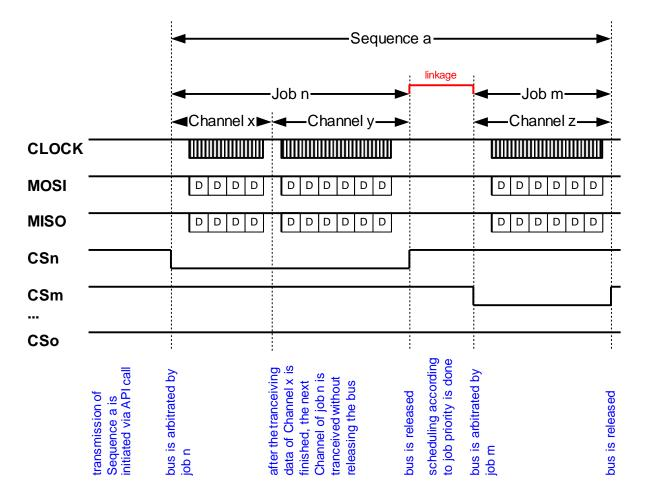
Channel data may differ from the hardware handled and user (client application) given. On the client side the data is handled in 8, 16 or 32bits mode base on SpiDataWidth (see chapter 8.2.5). On the microcontroller side, the hardware may handle between 1 and 32bits or may handle a fixed value (8 or 16bits) and this width is configurable for each Channel (see SpiDataWidth)..
