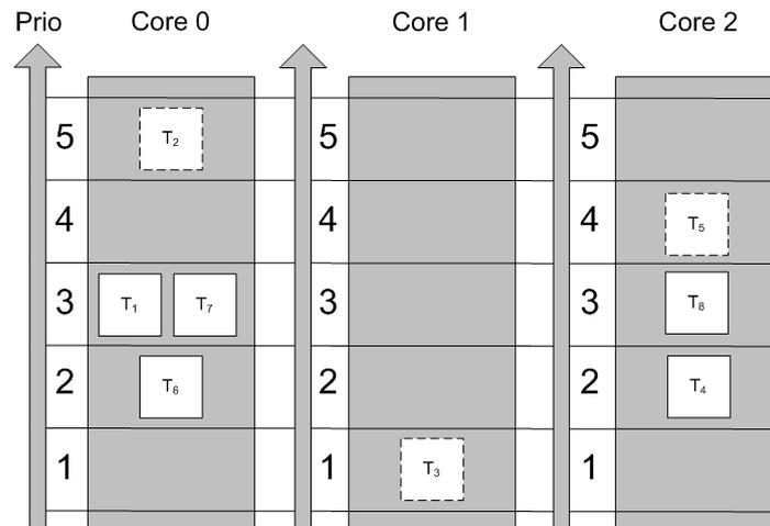
**Figure 2: Priorities are assigned to TASKS. The cores schedule independently from each other. The TASKS T<sub>2</sub>, T<sub>3</sub> and T<sub>5</sub> are executed in true parallelism. TASKs with the same priority on the same core will be executed in order of activation; TASKs with the same priority on different cores may not be executed in the order of activation, since the cores schedule independent from each other.**
