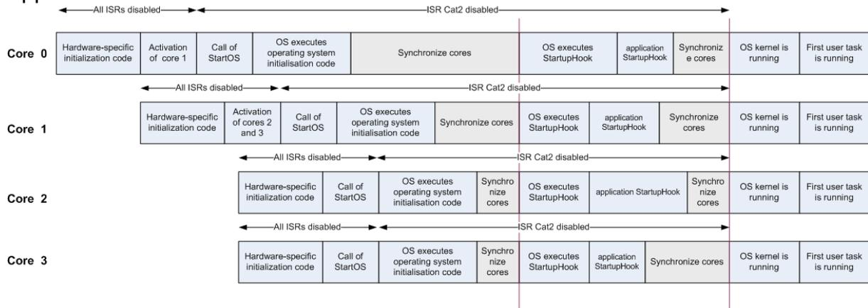
Figure 3: This figure shows an example of an initialization process with 4 cores.
