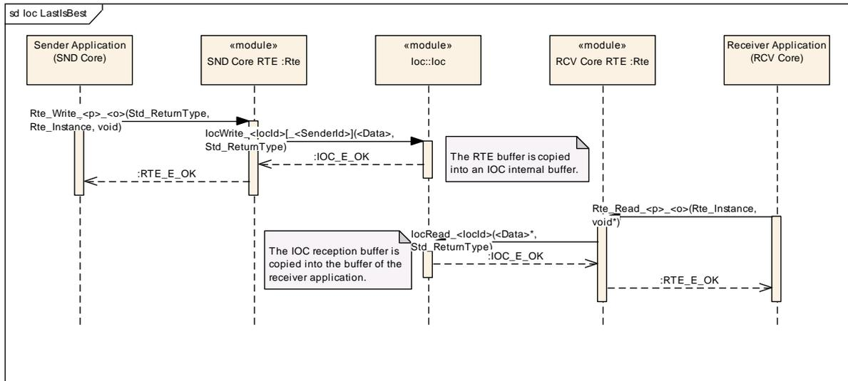
**Figure 12: IOC - LastIsBest communication**
