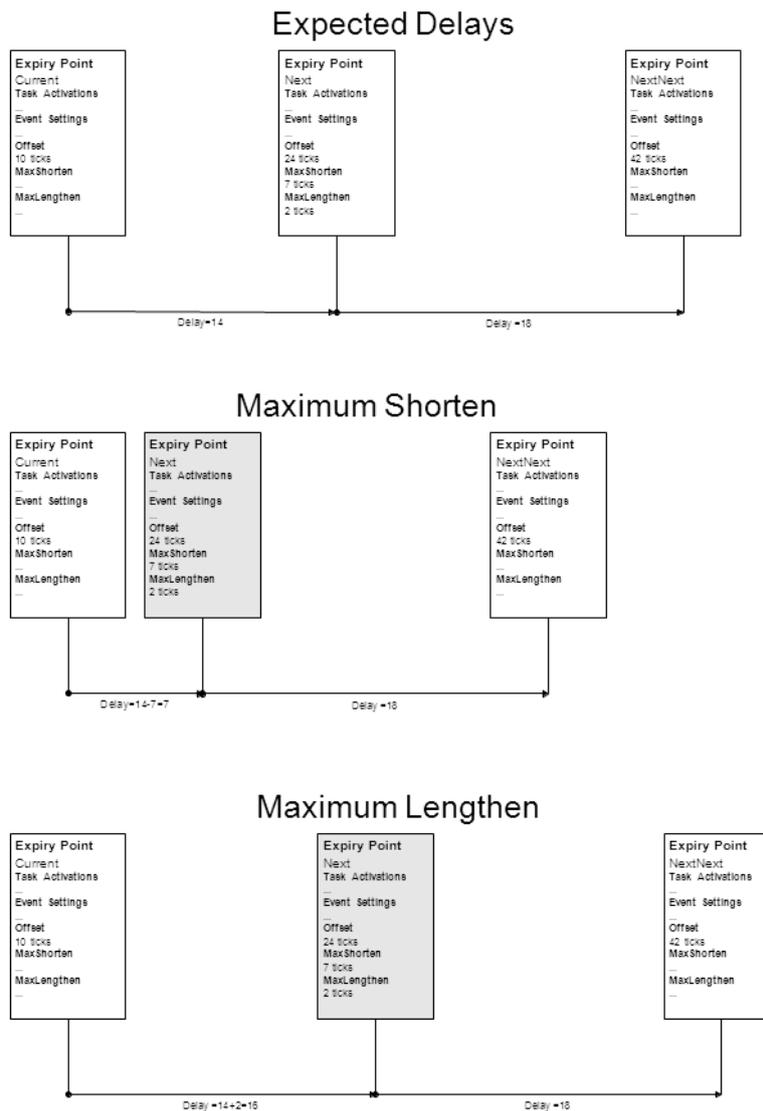
**Figure 7.7: Adjustment of Expiry Points**
