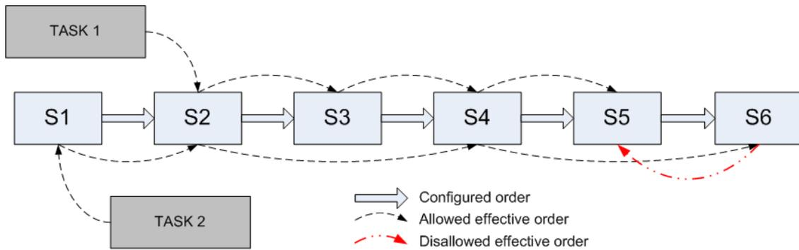
**Figure 9:** This figure shows an example in which two TASKS have access to a set of spinlocks S1 -- S6. It is allowed to occupy the spinlocks in the predefined order and it is allowed to skip spinlocks. If multiple spinlocks are occupied at the same time, locking and unlocking has to occur in strict LIFO order.
