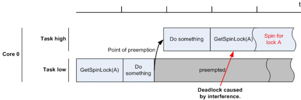
**Figure 7: A deadlock situation caused by interference, the high priority TASK spins indefinitely because the low priority TASK has occupied the spinlock. In such cases the second GetSpinlock call will return with an error**
