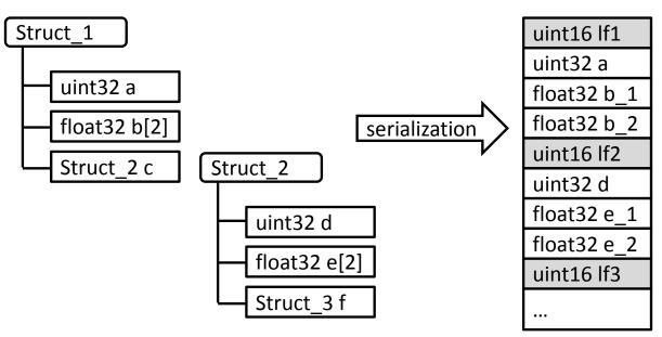
Figure 7.5: Serialization of Structs with Length Fields (Example)
