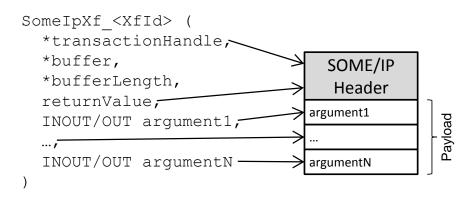
Figure 7.12: Example for serialization of a Client/Server Response
