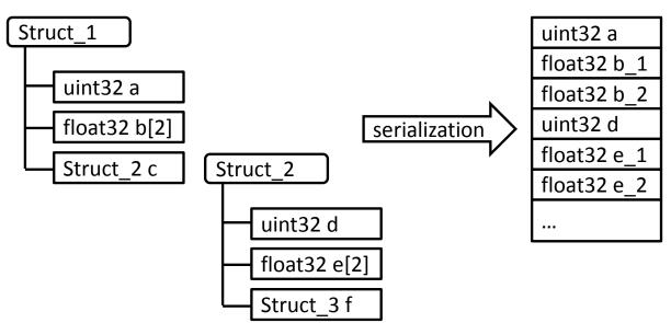
Figure 7.4: Serialization of Structs without Length Fields (Example)
