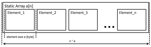
Figure 7.7: One-dimensional array (fixed length)
