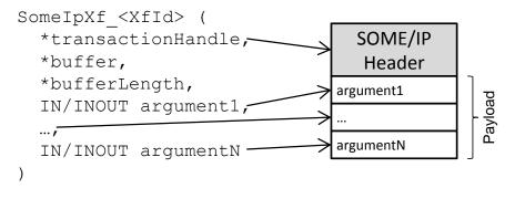
Figure 7.11: Example for serialization of a Client/Server Request
