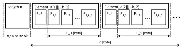
Figure 7.10: Multidimensional array (dynamic length) (Example)
