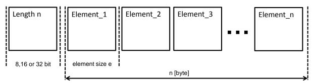
Figure 7.9: One-dimensional array (dynamic length) (Example)
